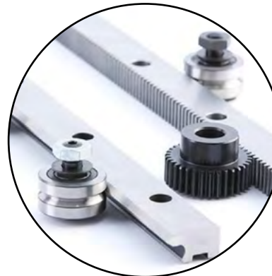
HepcoMotion linear guides for contaminated environments. The V guide and rollers provide a self-cleaning action that expels dust and abrasive concrete particles, preventing them from entering the rolling contact zone.
